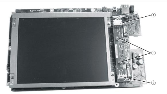
1. LCD Backlight Cable, permanently attached to LCD Assembly.
