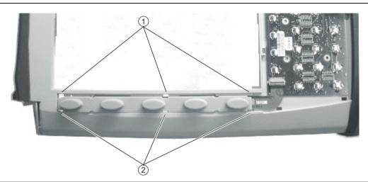
1. Location of three (3) upper locking tabs on the Soft Key Keypad Bezel (not shown) and the Keypad Membrane. 2. Location of three (3) lower locking tabs.
