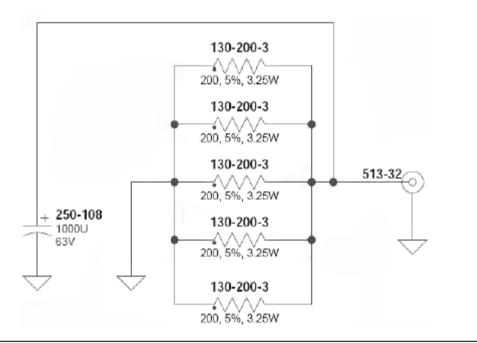
Figure B-1. T2904 Test Fixture Schematic
