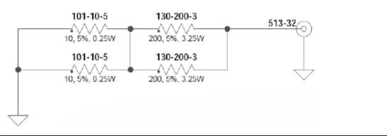
Figure B-2. T3377 Test Fixture Schematic
