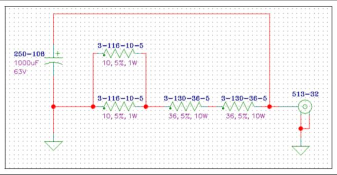
Figure B-3. T3536 Test Fixture Schematic
