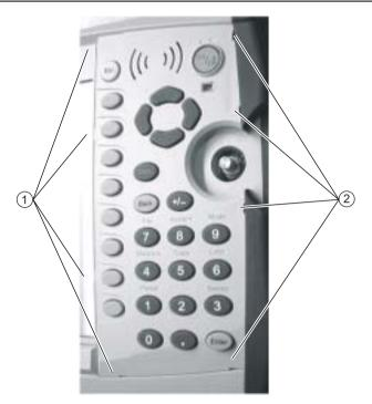
1. Location of four (4) left side locking tabs on the Main Keypad Switch Bezel.
