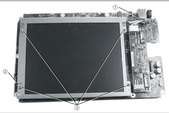
LCD Backlight Cable, permanently attached to LCD. Connects to Backlight Power Inverter Assembly.
