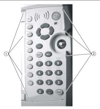
1. Location of Main Keypad Switch Bezel four (4) left side locking tabs 2. Location of four (4) right side locking tabs.
