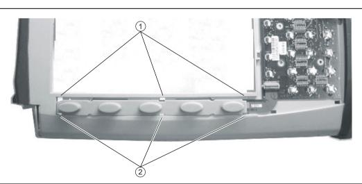
Location of three (3) upper locking tabs on the Soft Key Switch Bezel and underlying Soft Key Membrane.
