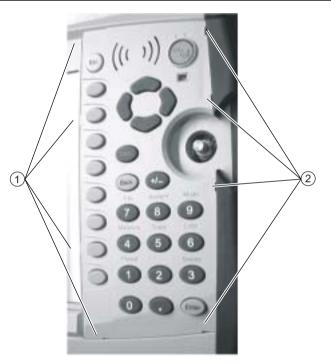
Location of four (4) left side locking tabs on the Main Keypad Switch Bezel.
