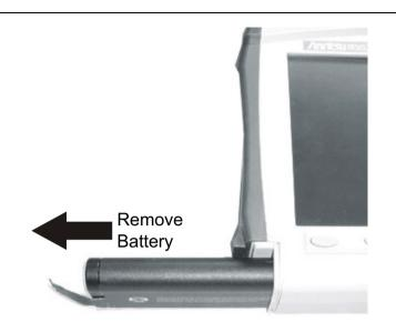
Figure 3-4. Removing the Battery
