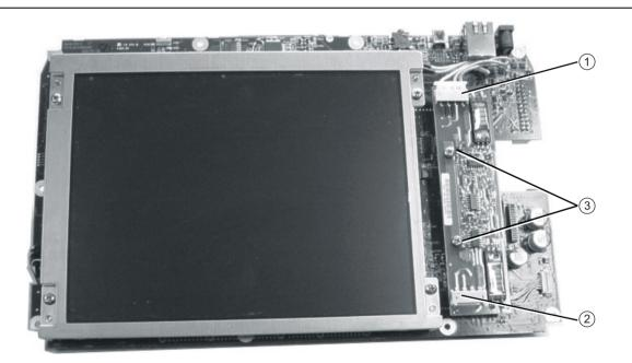
LCD Backlight Cable, permanently attached to LCD. Connects to LCD Backlight Power Inverter Assembly.
