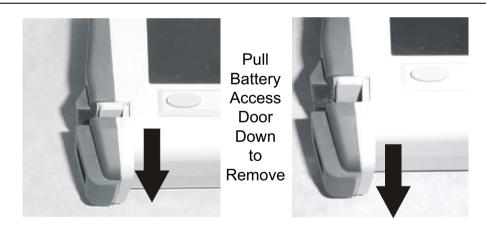
Figure 3-3. Removing the Battery Access Door
